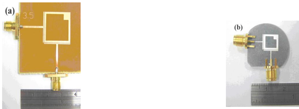
Fig. 2 Photograph of the filter prototypes: (a) FR4, and (b) NMTB ceramic substrates.
