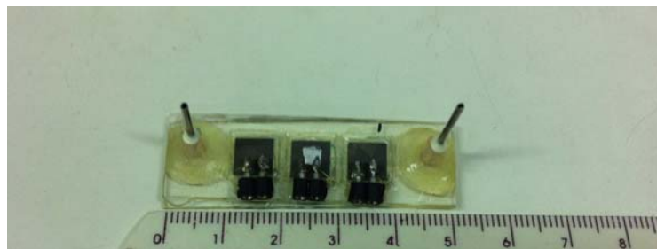
Fig.3 Completed UV adhesive based peristaltic micropump
